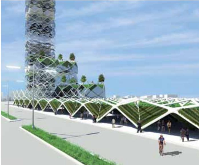
Middle: The Seawater Vertical Farm by the Venice-based studiomobile uses seawater, sunlight and passive solar energy to cool and humidify air and produce fresh water to grow plants. Envisioned for Dubai, it addresses the region's lack of fresh water and vegetables, and also promises to increase the water evaporation in the areas surrounding it, creating a cooler and more humid micro-climate.
